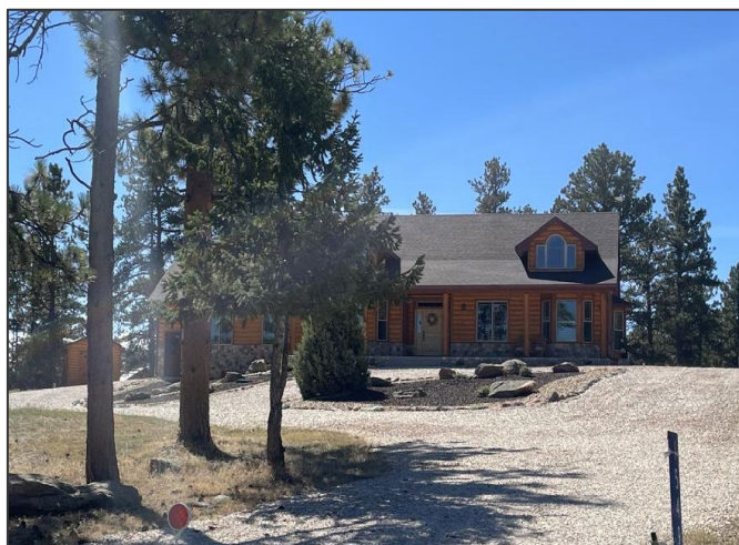
Some homes in the GVFPD have exemplary defensible space: mowed grass near structures, trees limbed and not overhanging roofs, and non-flammable barriers out to 5 feet from the home. Photo credit: TEA.
